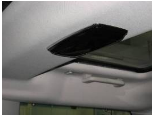
WhiteFire™ emitter mounted in the roof headlining. Self coloured gloss black lens.
