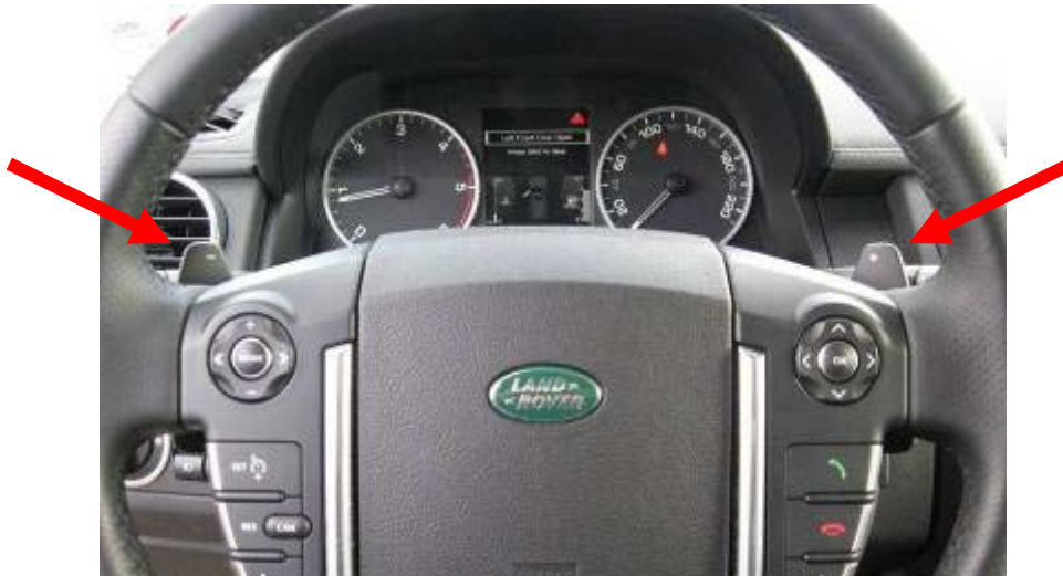
Steering wheel mounted gearshift paddles (arrowed) on 8-speed diesel derivatives
