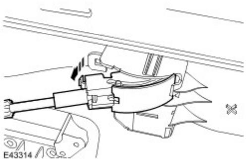
5) Remove the door trim by disconnecting the electrical connectors including puddle light. It may be easier if you leave the electric window connector until last.
