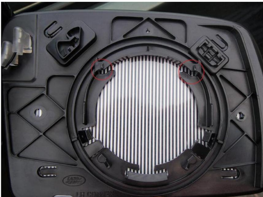
You then need to push the glass in and down to secure. This was the tense moment as too much pressure and the glass could break.
