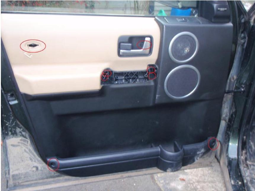
3) Using a flat screwdriver or piece of plastic, prise the panel away from the door. I started from the bottom and worked around the left hand side then the right hand side. Finally, I pulled the panel away from the door from the top left and worked across to the speaker on the right hand side. The bottom and sides are secure by 12 plastic lugs (4 on the each side and 4 at the bottom) where as the top is secured by 5 metal clips.
