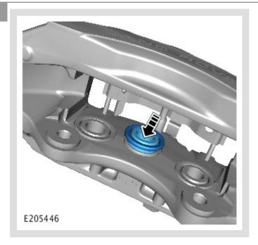
Carefully push the caliper dust boot and the caliper piston partially into the caliper bore. Make sure that there is no damage to the piston surfaces during this installation.
