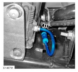
31. Connect the new air line link pipe.
