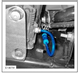
14. Connect the new air line link pipe.
