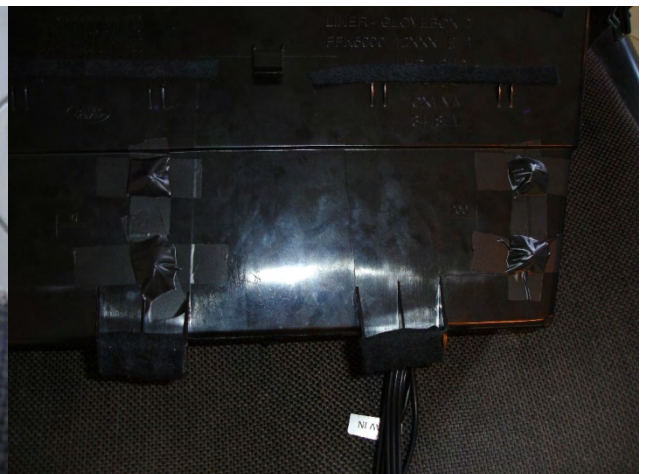
(screw tips covered with tape – underside of glovebox)
