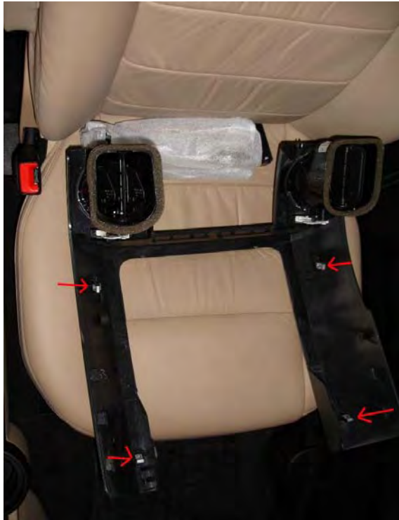
(this is where the clips should be, they're on now)
