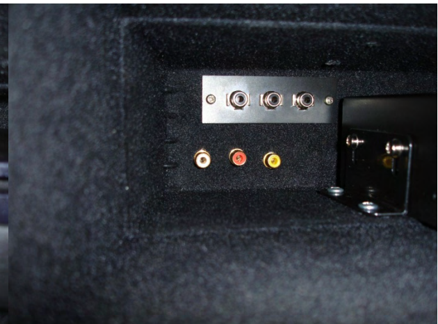
(...and RCA plugs fitted)
