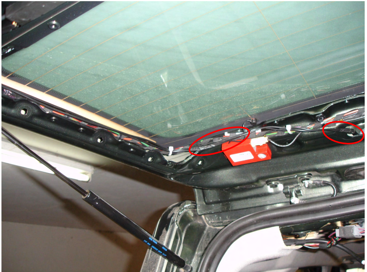
(highlight of potential chaffing spots – add thickness by means of electrical tape)
