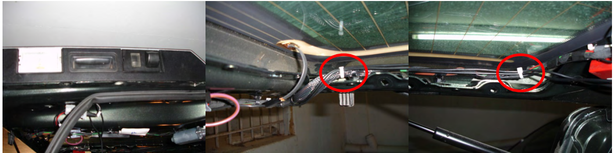
(cables and gasket clear of bodywork...) (...cable routed to lower left corner...) (...and upper left corner)
