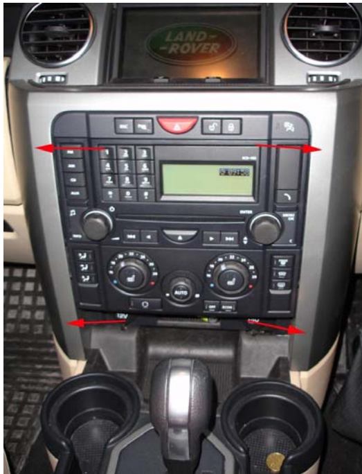
(H-panel in place...)
