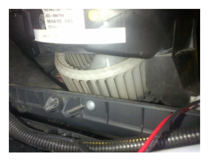
Below is one of the AC water drains that can come disconnected from the AC ducting nipples and hence "wet the carpet". There are two of them, the other being on the driver's side. The rubber just shrinks by itself, disattaches, and instead of the water flowing thru the floor boards onto the ground, it soaks into the carpet. It is not only AC condensation water but also rain or car wash water that can get into the system and hence is supposed to flow thru the drains.
