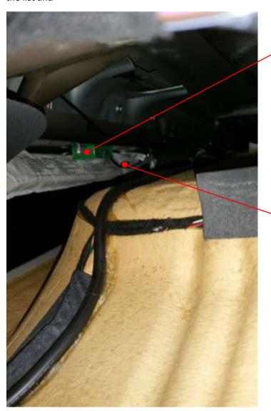
Antenna interface — (FM/DAB Receiver) in place, this is actually my original unit, I fitted a grey unit in it's place, one screw, one connection onto the glass
