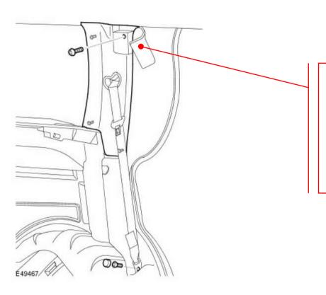
Remove this trim access cover and remove the Torx screw.
