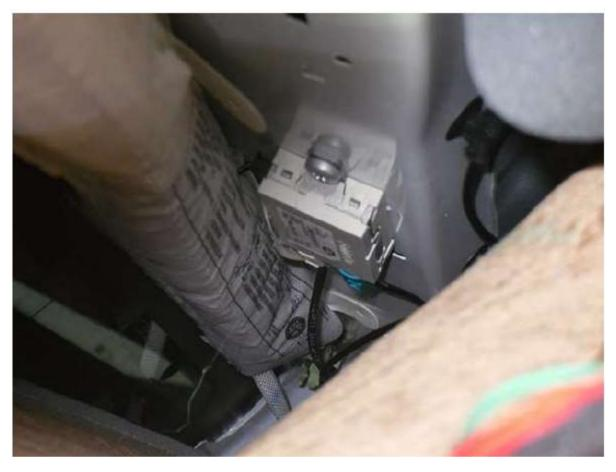
Put some tape on the antenna cable and attach it to the existing loom that runs around the perimeter of the headlining, don't leave it loose, you just know it will rattle against something and it will give you the shits!, I used some duct tape (cloth tape 50mm wide, very aggressive adhesive) to secure the antenna cable up the "C" pillar and onto parts of the underside of the headlining where I could not get at it easily.
