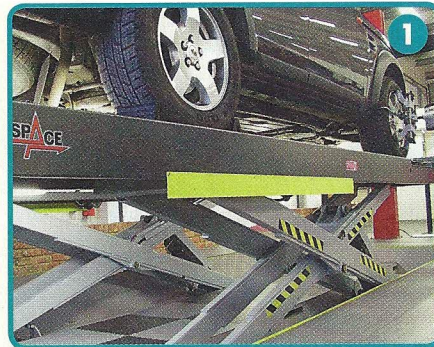
1 Sophisticated vehicle lift provides accurate level platform, up-lighting, and suspension-play detector, which we'll see in action later
