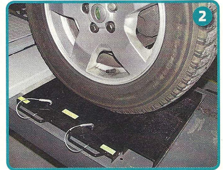
2 These turntables on the platform allow the wheels to move without deforming the tyres, which would affect the measurements
