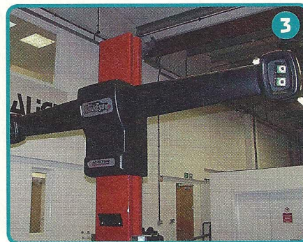
3 This sophisticated imaging sensor column at the head of the vehicle platform carries two digital cameras at the end of each arm
