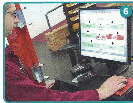
6 The technician's monitor shows geometry, manufacturer specifications, effects of adjustment and predicted error symptoms...
