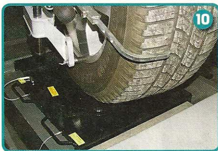
With the front wheels resting on turntables to avoid any tyre flex affecting the readings, the steering is turned from lock to lock
