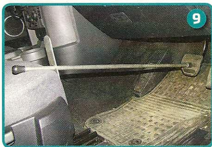
First, the front castor angle is checked. Brake pedal is clamped down to eliminate any hub bearing play from readings
