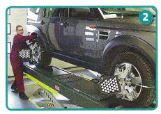
The vehicle is then manually rolled back while the cameras track any wheel rim runout as the targets revolve with the wheels
