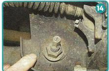
This is the nut and washer on the front fork to chassis. The camber bolt is turned to move link in or out to adjust camber
