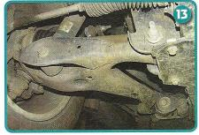
Front lower wishbone arm is located to chassis by camber bolts, washers and nuts at the end of each fork of the wishbone
