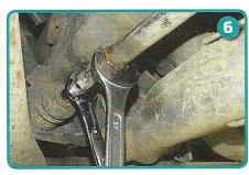
Toe is adjusted by screwing the inner rod into the tubular link, similar to adjusting the front toe on the steering track rod
