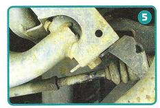
It engages a screwed rod at its inboard end, which connects to the chassis via a rotational joint (which is concealed by the rubber gaiter)
