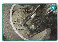
Starting at the rear axle, individual wheel toe is adjusted on the tubular transverse link (bolted and bushed to the hub/knuckle)
