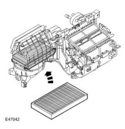
The cabin air filter is installed in the air inlet duct and is either a pollen filter or a pollen and odor filter. The pollen filter removes particulates, and the pollen and odor filter removes particulates and unpleasant odors, from the fresh and recirculated air entering the blower.
