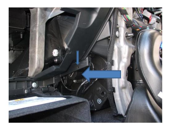
Arrowed in the next photo is roughly where the upper (footwell and face) motor is. Access to this involves removal of the plastic ducting.
