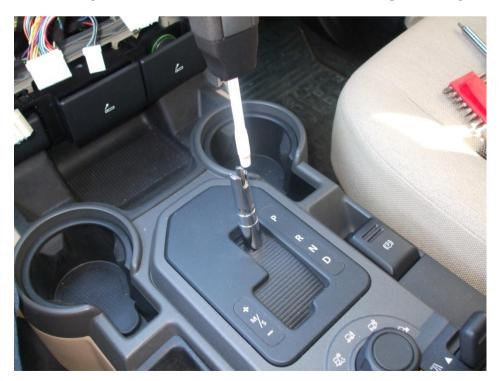
14. Remove the Torx screw from just in front the EPB handle.
