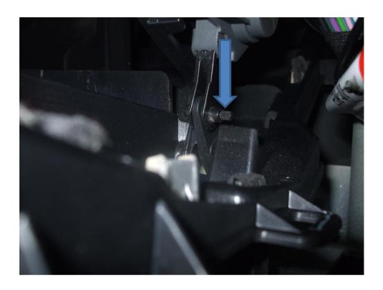
11. Then push inwards the hinge pins on both sides. The right one needs varying lengths of stiff wire.
