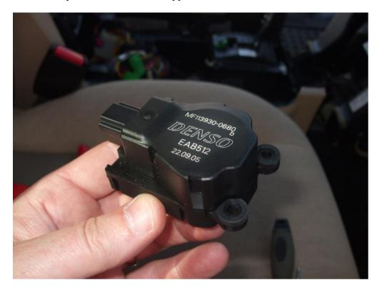
26. From what I found out by trial and error, there's four of these little guys hiding away. There are two on the left (passenger side) – the bottom one (big arrow) does the passenger side temperature mix, the top one controls the air flow between the footwell and the face vents.
