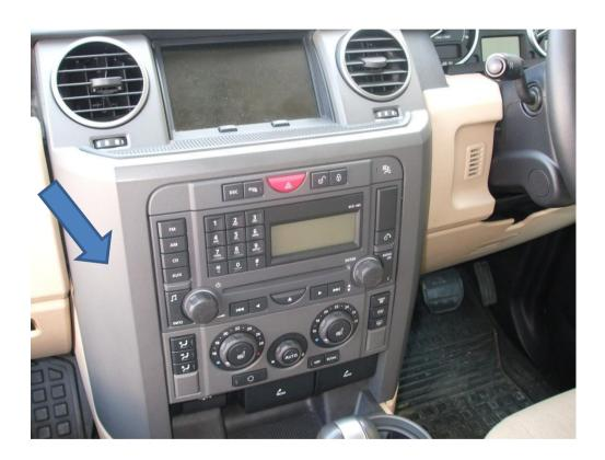
5. Remove the satnay, stereo and heater controls etc. Be careful of some of the connections at the rear, especially the optic fibre ones. Note that the bottom one, the ashtray and 12v sockets won't come out yet.
