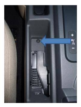
Now pull the top section of the console upwards. A lot of plastic breaking sounds will be made that sound expensive. At least one clip of mine is permanently broken. I don't think there's any trick here, just luck.
