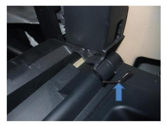
10. Looking inside (where the satnav once was), find the mechanism that dampens the opening of the glovebox door. Move it to a point where you can see as shown below (the pin won't be half out... you need to do this) and push it from the left-hand side with a small screwdriver etc. Don't push out too far or else it's goodbye to the pin. Pull out the remainder of the way with long-nose pliers.
