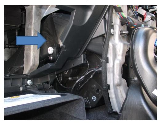
27. Here's the right (driver's) side. Again, the lower one (large arrow) does the driver's side temperature mix. The upper one (completely hidden from view by plastic ducting) does the windscreen and side window (the ones that can't be opened/closed) vents.
