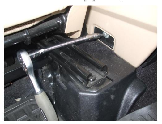
13. If you have an auto like me the next bit is relevant. If you have a manual, sorry, I haven't got a clue. Hold the gear selector handle and pull upwards... hard... but straight in line with the lever so as not to break the plastic bit goes downwards inside.
