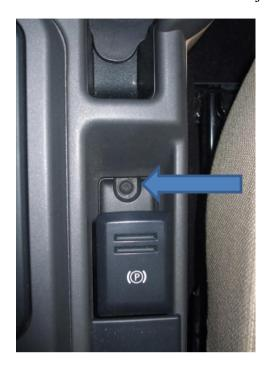
15. Remove the rubber sunglasses holder, and the plastic bit underneath it. A hidden Torx screw should be found underneath. Very cunning.
