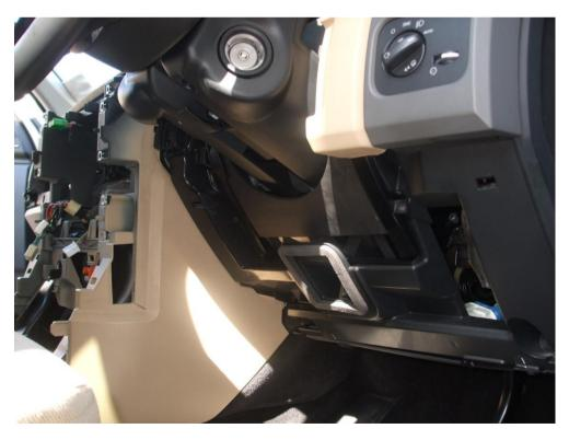
22. Squeeze the stays on either side of the lower glovebox when open, so it drops down to its lowest position.
