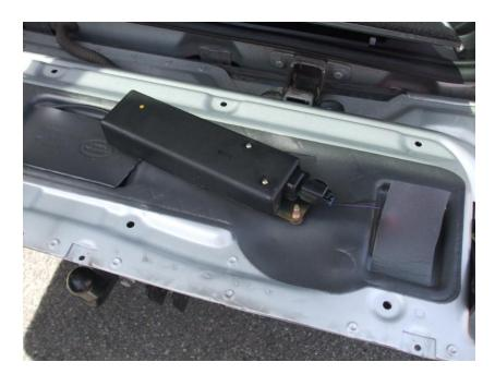
Remove the plastic cover by (two Torx screws). When the actuator operates the cable is pulled in the direction of the arrow
