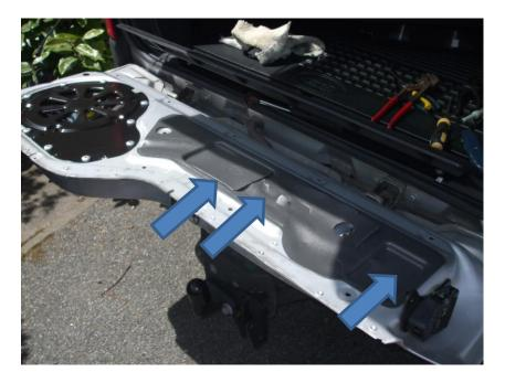
Partially loosen these two nuts. They are on keyhole slots so one or two turns is fine, no need to remove
