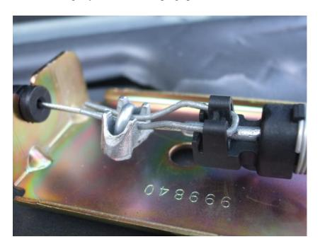
A cable tie around the wire ends, and bending of the loop to tighten it up a bit
