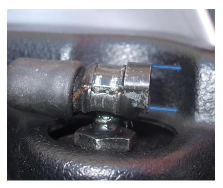
Remove the ball joints with a deep socket. The female thread is part of a metal bracket and therefore there's no nut etc to lose
