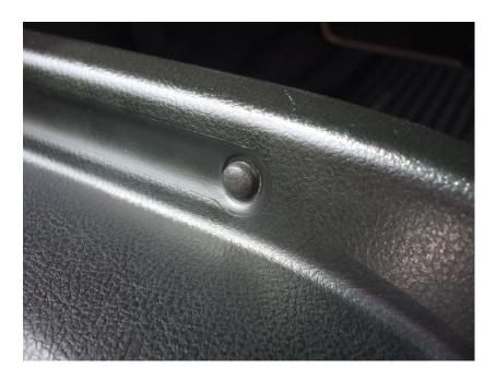
Remove the four pozidrive screws. The trim needs to be removed; open the tailgate and insert a large flat-blade screwdriver under the trim close to where the four screwholes are. Tap the end of the screwdriver handle and the trim should release and pop off. Work along the trim pushing the screwdriver under the trim in the four locations of the screws
