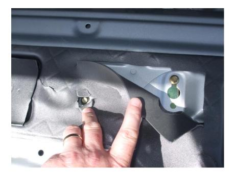
The actuator has to be removed through the large hole on the left (nearside), having first removed the electrical plug via the right-hand hole. The plug and socket are arrowed below
