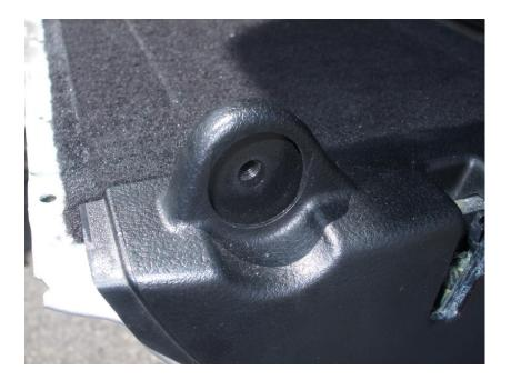
Pop the carpet off, there's ten clips around the circumference, the top edge can be prised up with a large screwdriver, the bottom can be pulled up.
