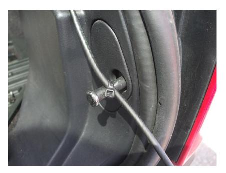
Slide the clip holding the end of the cable on the ball joint. Once at about the position shown below the socket should come away from the ball. Do this on both cables. Ensure that the weight of the tailgate is adequately supported to avoid damage – remember now that any downward pressure will have to be supported by what's been placed between the tailgate and the bumper
