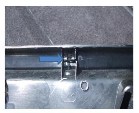
The carpet panel from the rear of the tailgate now needs to be removed. This involves disconnecting the supports on each side; because of this the tailgate will have nothing to take its weight. One solution is to place something soft on top of the bumper; an old rolled up bathmat was used here
