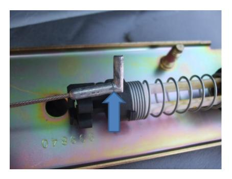
Cable refitted, bend a length of wire through the plastic clip from the wire cable and back around to it
