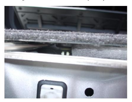
There are five clips along the top edge and five along the bottom. When prising or pulling up, try to pull up where there's a clip
