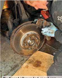
The disc and caliper go back on and, once both are bolted up, Rob checks that the disc turns cleanly by rotating it a couple of times.
