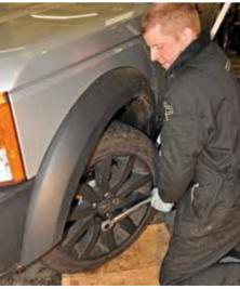
After replacing the wheel, there's no evidence of play; and a test-drive reveals a distinct lack of roughness from the nearside front wheel bearing. A successful outcome.
