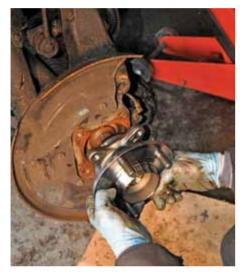
Disco 3 owners needn't worry about pushing out bearings or fret about pressing replacements in straight, because the job has been somewhat dumbed down to a straight swap of the complete hub and bearing assembly. So, making the actual repair is the quickest and easiest part of the job. This ease of replacement does sugar the pill of the assembly's £100 price tag a little.
