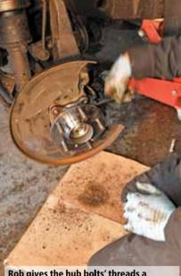
Rob gives the hub bolts' threads a coating of copper grease and tightens them gradually to bring the hub's flange in good and square.
