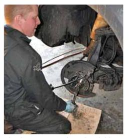
A brand-new nut is screwed on to the end of the driveshaft and is torqued up to 230Nm. This stake nut has a ring that is punched down into a groove in the driveshaft to prevent it from coming undone. It's common to see these straightened out and re-used, but the metal is then much weaker (having been work-hardened) and the potential for the nut coming loose is higher.
