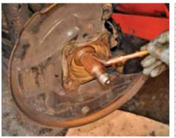
Coating the driveshaft in copper grease will ensure that it won't stick to the driveshaft and will make any future repair here much easier.
