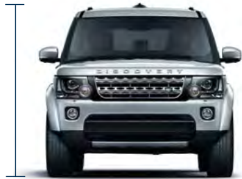
Front wheel track 1,605mm
