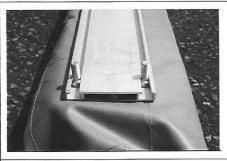
Now that the brackets are in place, you need to put the remaining 4 M6 bolts into the groove of the backside of the awning.
