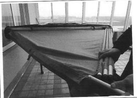
All poles are hinged and telescopic. They lock and unlock with a slight twist. Unfold the horizontal poles.
