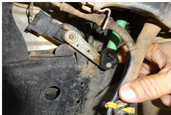
Figure 4: Swapping fronts to new position. Note front set-up for RRS is shown (D4 is reversed)
