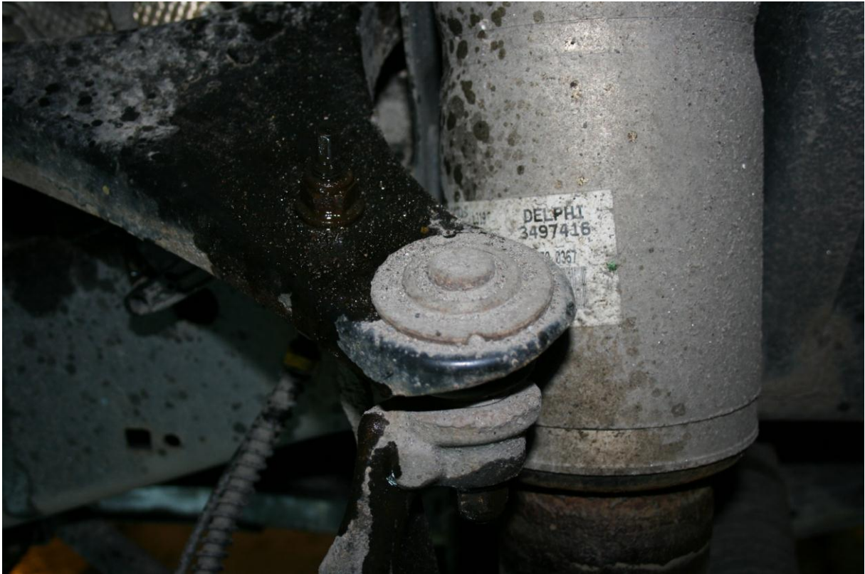
Then started on the actual job. Loosened ARB link, and the ball joint.
