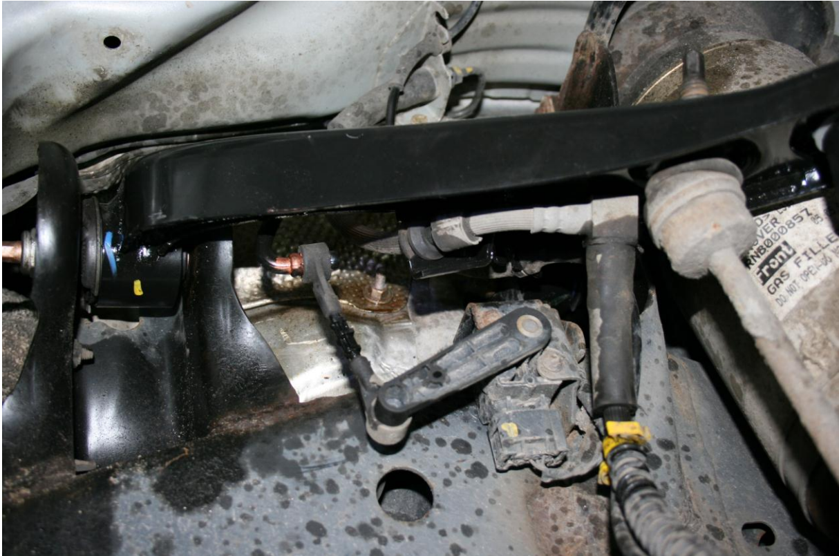
New arm in place. The ARB link were replaced later, just here to hold the arm up. All bolts were sprayed with copper grease before replaced. Loosely fastened
