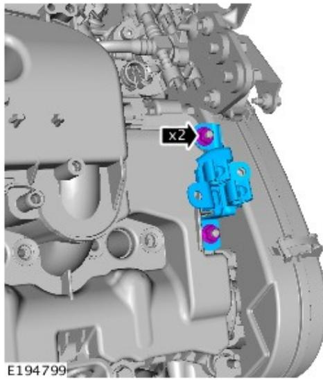
Remove the left valve cover mounting bracket.
