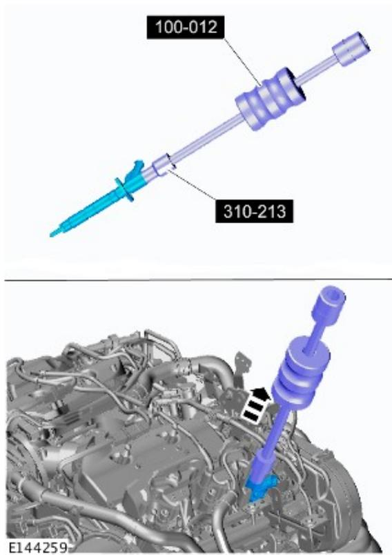
Using the special tools remove the fuel injector.
