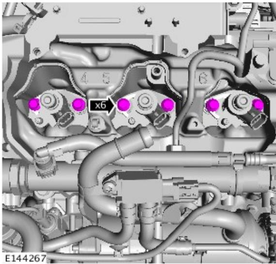
Remove the fuel injector bolts.
