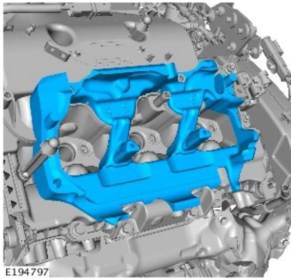
Remove the Noise, Vibration and Harshness material.
