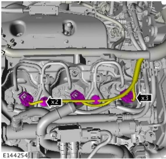
Disconnect and release the fuel injector wiring harness.
