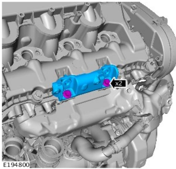
Remove the fuel rail mounting bracket.
